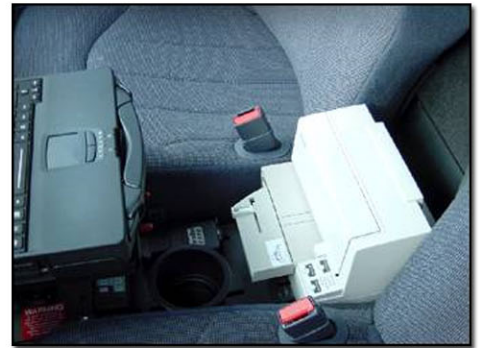
Inside the patrol car, a laptop and ticket printer automates -- and expedites -- the filling out of tickets.
